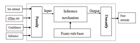
Figure 1. Structure of Fuzzy Rule-based Systems [14]
