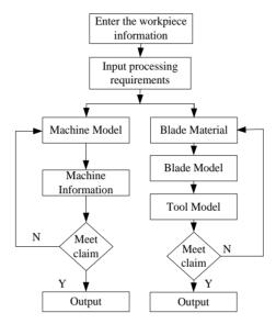
Figure 2. Flowchart of Interactive Preferred of Machine and Tool
