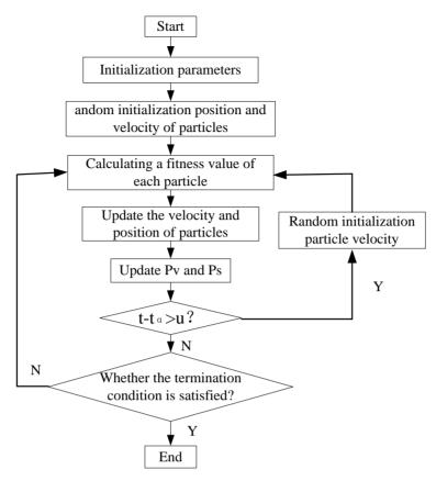
Figure 3. Flowchart of PSO Principle
