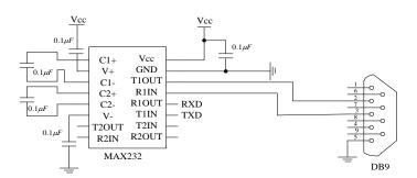
Figure 4. The Serial Communication Circuit based on MAX232
