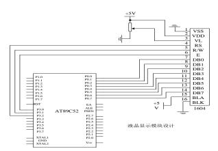
Figure 6. The Wiring Diagram of LCD and AT89C52
