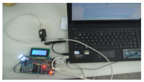
Figure 10. The Actual Operation Condition of the Color Analyzer
