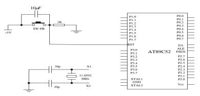
Figure 3. The Wiring Diagram of the Reset Circuit and the Crystal Circuit
