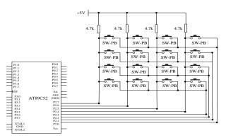
Figure 5. The wiring Diagram of the Matrix Keyboard Interface and AT89C52
