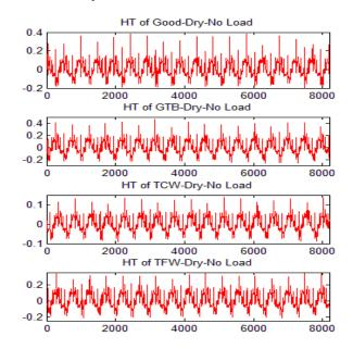
Figure 6a. Hilbert Transform Plot for Dry Lubrication and No Load Condition
