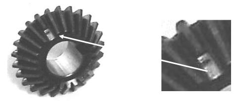
Figure 4. (c) View of Pinion Wheel with Tooth Breakage (GTB)
