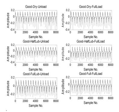
Figure 5. Vibration Signal for Good Pinion Wheel under Different Lubrication and Loading Conditions
