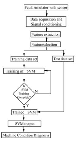
Figure 1. Flowchart of Fault Diagnosis System
