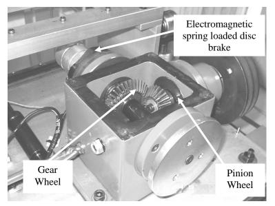
Figure 3. Inner View of the Bevel Gear Box
