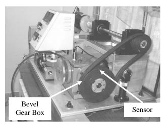
Figure 2. Fault Simulator Setup
