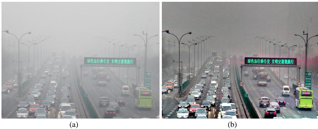
Figure 2. Hazy Image and the Result of MSR: (a) Hazy Image; (b) Result of MSR
