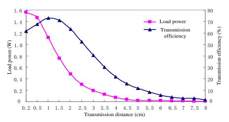
Figure 8. The Relationship Diagram among Transmission Distance, Load Power and Transmission Efficiency
