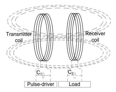
Figure 1. The Diagram of the Wireless Power Transmission System
