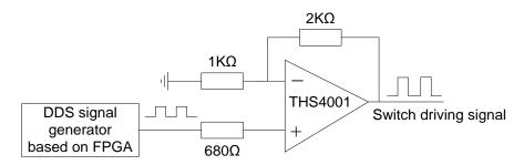
Figure 3. Diagram of Switch Driving Circuit
