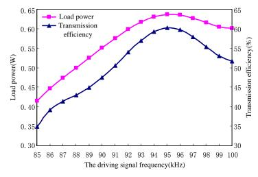
Figure 6. The Relationship Diagram among the Driving Signal Frequency, Load Power and Transmission Efficiency
