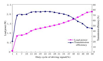
Figure 7. The Relationship Diagram among Duty Cycle of Driving Signal, Load Power and Transmission Efficiency
