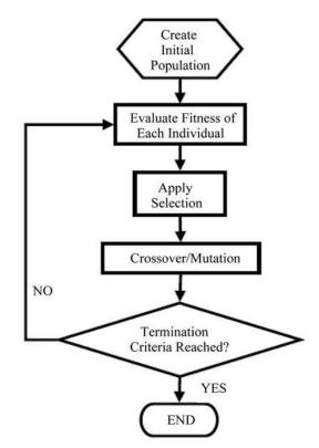
Figure 4. Processing Flow of GA
