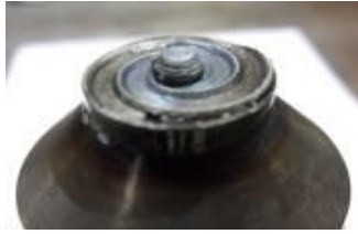
Figure 1. FSW Tool with a Scrolled Shoulder a Threaded Conical Pin
