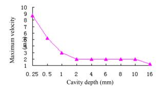
Figure 8. Influence Curve of the Oil on the Maximum Velocity
