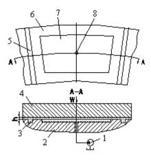
Figure 1. Constant Flux Oil Supply System of Hydrostatic Thrust Bearing 1pump, 2-guide rail, 3-Interstitial Fluid, 4-rotary Table, 5-return Chute, 6-land, 7oil Pocket, 8-fuel Feed Hole, w-external Load, h-oil Film Thickness
