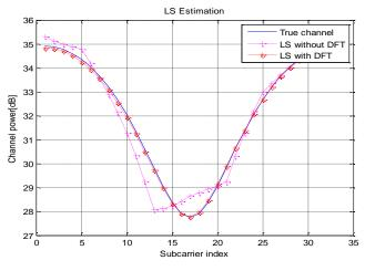
Figure 4.1 LS estimation with & without DFT
