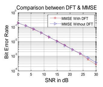
Figure 4.4 BER VS. SNR comparison between DFT and MMSE estimation
