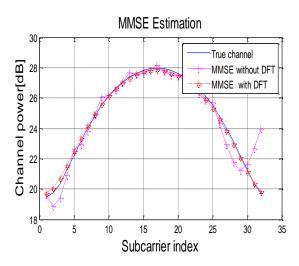
Figure 4.3 MMSE estimation with & without DFT
