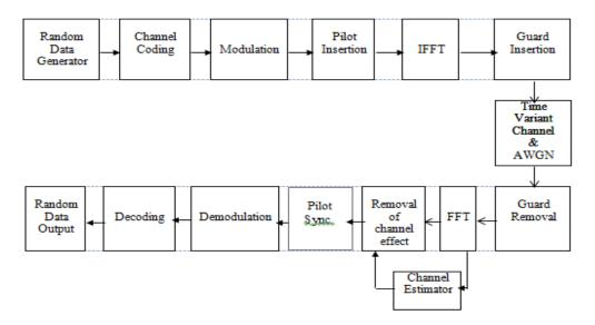
Figure 2.3.Block diagram of OFDM system with channel estimator
