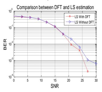
Figure 4.2BER VS. SNR comparison between DFT and LS estimation.
