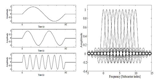
Figure 2.2.The real parts of three of the basis functions (Left) and the concept of densely packed subcarriers in OFDM (right)
