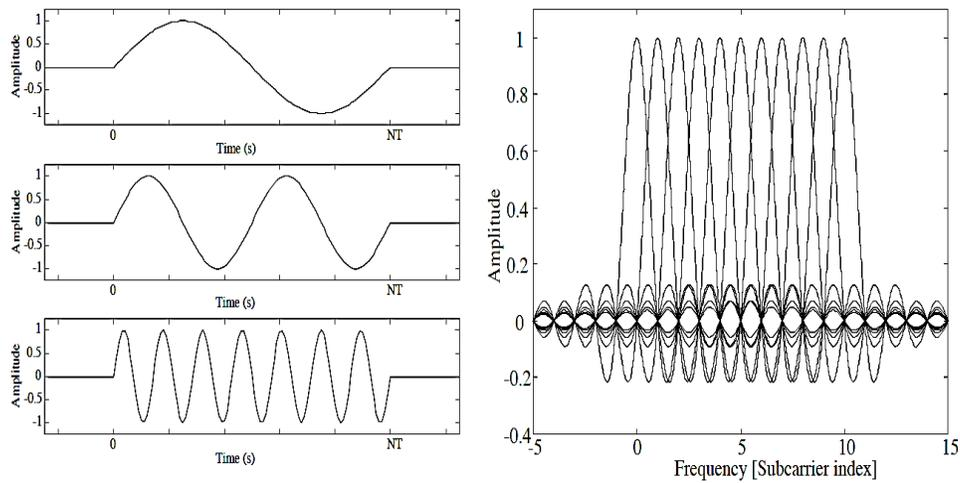
**Figure 2.2. The real parts of three of the basis functions (Left) and the concept of densely packed subcarriers in OFDM (right)**
