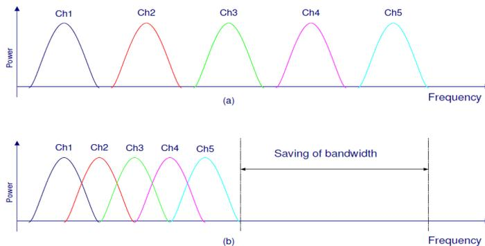
**Figure 2.1. (a) FDM system (b) OFDM system**
