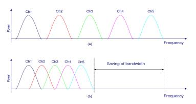
Figure 2.1. (a) FDM system (b) OFDM system
