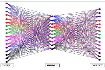
Figure 1. Neural Network with 17-input, 10-hidden, 15-output neurons
