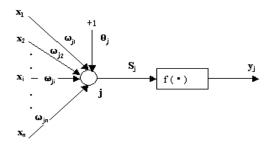
Figure 3. The structure of the artificial neuron
