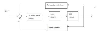
Figure 5. Edm machine servo control system block diagram
