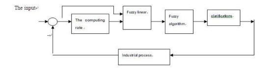
Figure 2. Fuzzy control system diagram
