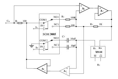
Figure 3. Digital Equivalent Capacitor Circuit
