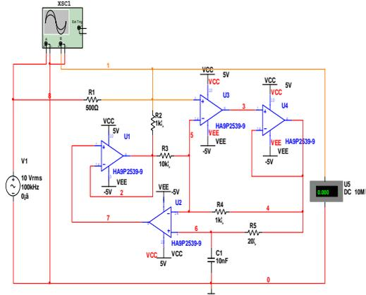
Figure 6. Equivalent Capacitance Simulation Circuit
