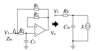
Figure 1. Equivalent Capacitor and Equivalent Circuit
