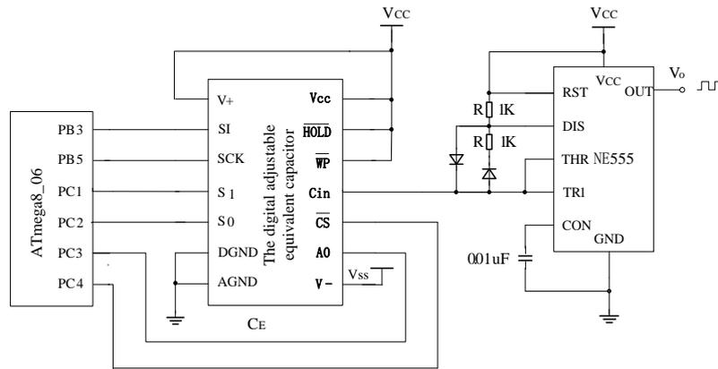
**Figure 9. The Multivibrator Consisting of NE555 Timer and Equivalent Capacitor**
