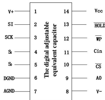
**Figure 4. Pins of the Digital Adjustable Equivalent Capacitor**
