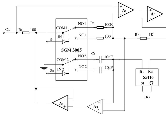
**Figure 3. Digital Equivalent Capacitor Circuit**
