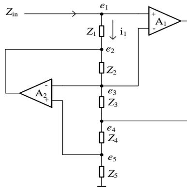
**Figure 2. Impedance Converting Circuit**
