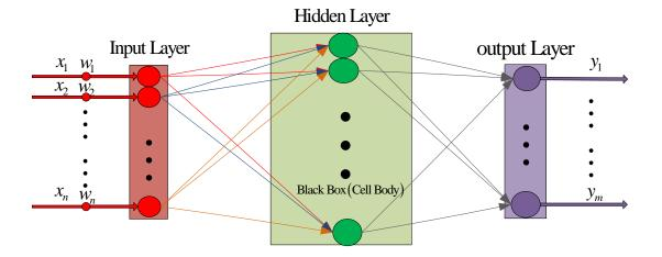
Here net<sub>j</sub> is the activation value of the *j*th node,  $y_j$  is the output of the hidden layer, and  $f_H$  is called as the activation function of a node, usually a sigmoid function can be described as follows:
