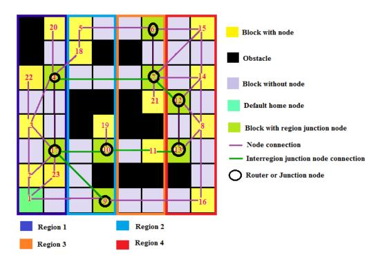
Figure 4. Robot Modified Path Map(RMPM)
