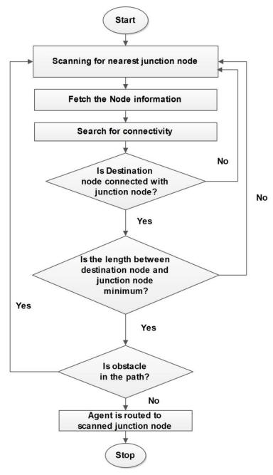
Figure 5. Modified Nearest Junction (MNJ) Algorithm
