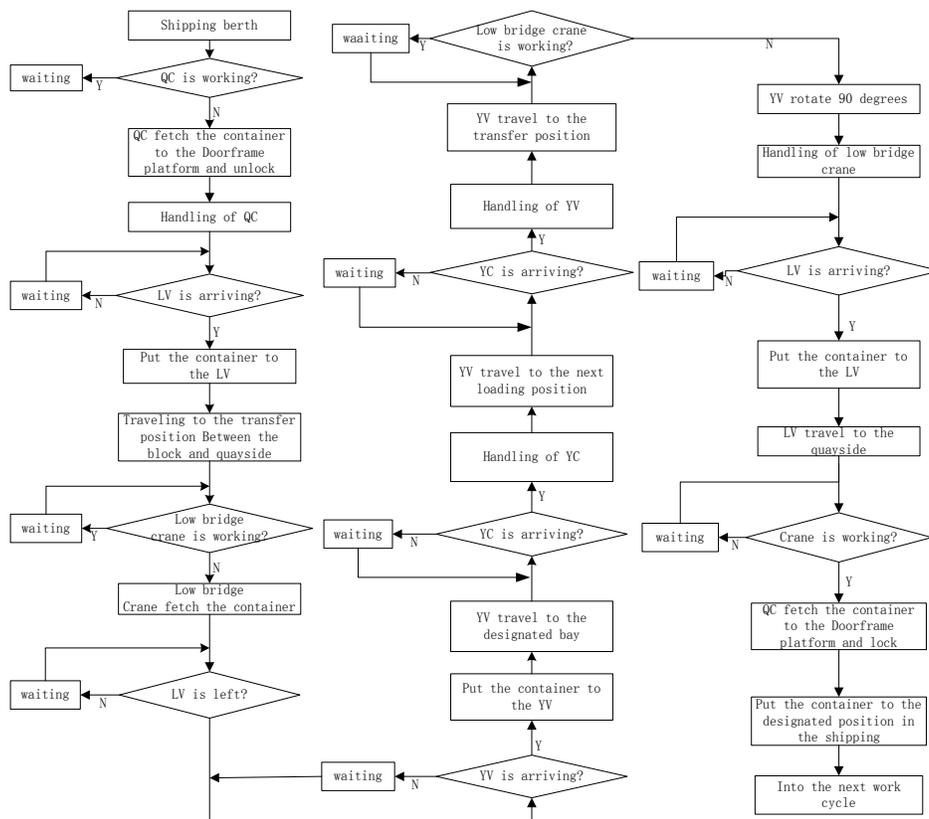
**Figure 3. Flowchart of loading and unloading**
