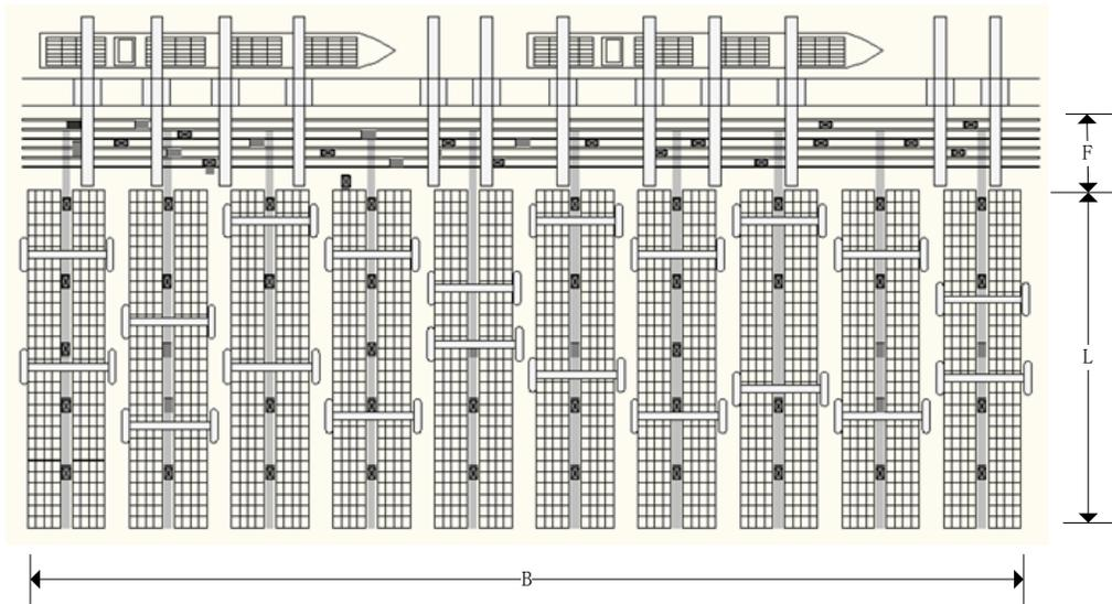
**Figure 2. Layout of container Terminal**
