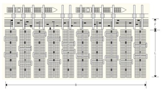
Figure 2. Layout of container Terminal
