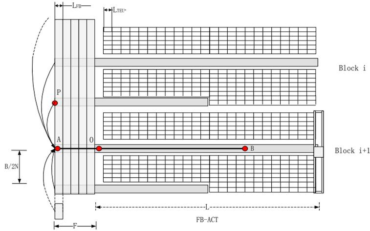
**Figure 5. The calculation of  $d_{YV}$  and  $d_{LV}$**
