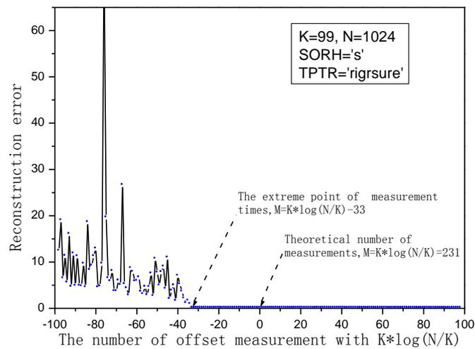
**Figure 1. The soft threshold reconstruction error**
