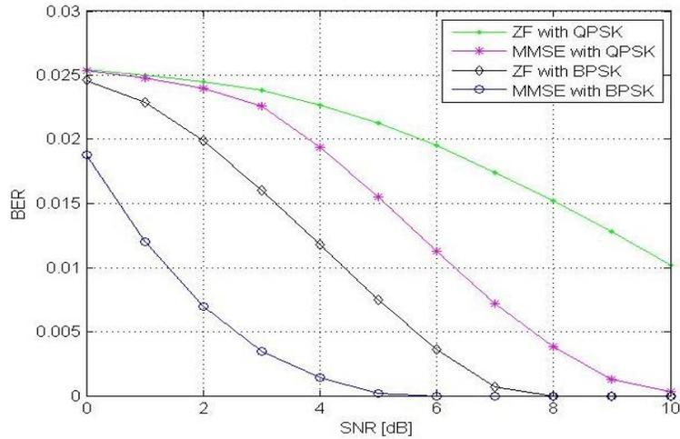
**Figure 2. BER performance of a convolutionally encoded and single relayed MIMO Cooperative OFDM wireless communication system with ZF and MMSE aided signal detection and various digital modulation schemes**
