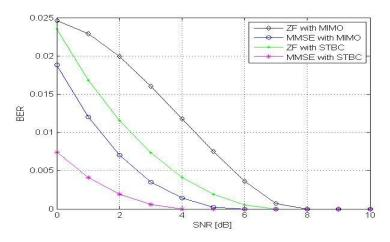
Figure 4. Plots BER vs. SNR of ZF and MMSE
