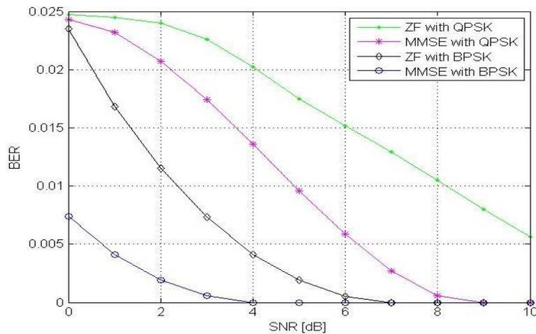
**Figure 3. BER performance of a convolutionally encoded and single relayed STBC based MIMO Cooperative OFDM wireless communication system with ZF and MMSE aided signal detection and various digital modulation schemes**
