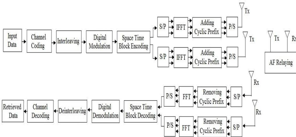
**Figure 1. Block diagram of Single Amplify and Forward Relayed Cooperative STBC encoded MIMO-OFDM system**
