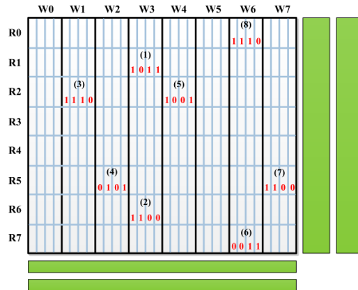
Figure 2. A faulty 8x8x4-bit memory
