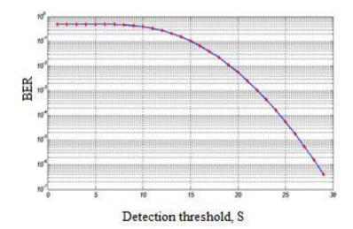
Figure 8. BER of code PC (25.5) with N=25 users as a function of the threshold of decision
