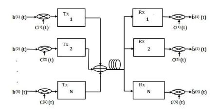
Figure 1. A transmission system DS-OCDMA
