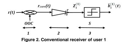
Figure 2 shows the principle of detection and estimation of the transmitted data, and which comprises 3 functions:
