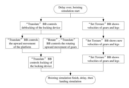
Figure 10. The simulation process of hoisting
