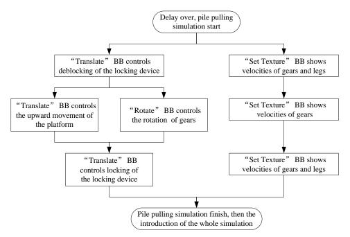
Figure 12. The simulation process of pile pulling
