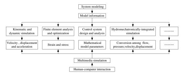
Figure 3. The procedure of integrated modeling for the virtual prototyping
