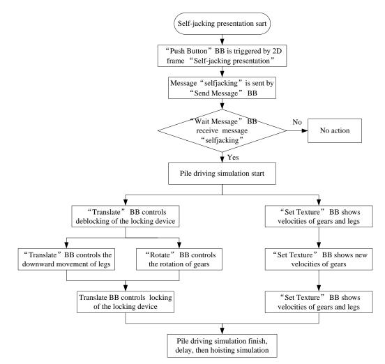
Figure 9. The simulation process of driving piles
