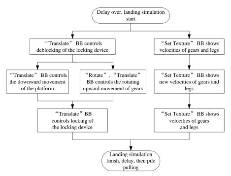
Figure 11. The simulation process of landing
