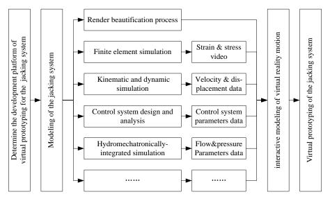
Figure 2. The overall design process of virtual prototyping for the jacking system
