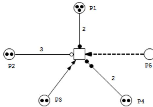
**Figure 4. Special arcs of  $SPN^C$  drawn in Snoopy, where the arc terminating with a small hollow circle is the inhibitor arc, the arc with a filled circle is the read/test arc, the arc with double filled circles is the equal arc, the arc with double arrowheads is the reset arc, and the arc with a dashed line is the modifier arc**
