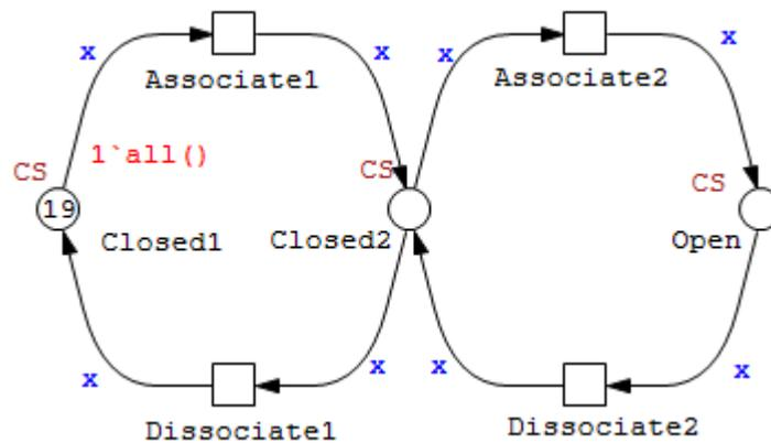
**Figure 3. A colored Petri net for the three-state model of a  $Ca^{2+}$  channel [26]. Declarations: colorset  $CS = int$  with 1-2; variable  $x: CS$ . This colored Petri net is obtained by folding two copies of the net in Figure 1**
