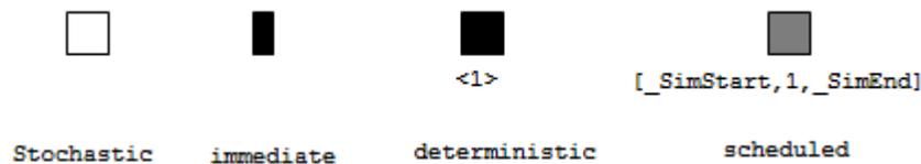
**Figure 5. Special transitions of  $SPN^C$  drawn in Snoopy**
