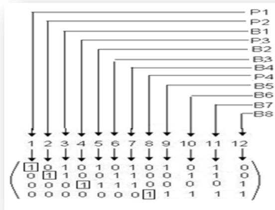
Figure 4. Locating the Positions for Insertion of Check Bits
