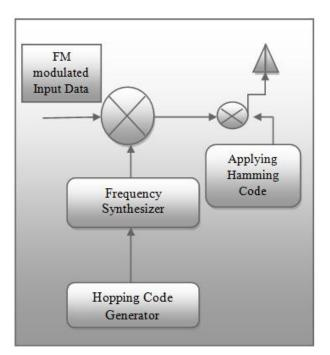
Figure 8. Transmitter for FHSS along Hamming Code
