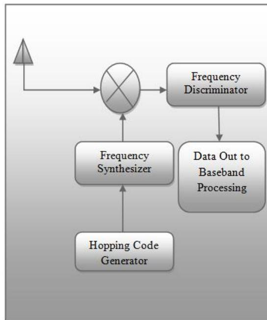
**Figure 2. Receiver for Frequency Hopping Spread Spectrum System**
