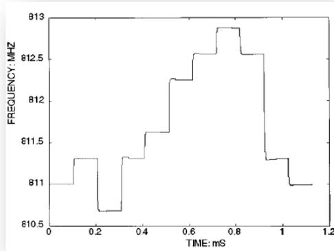
Figure 3. Frequency Hopping: Frequency Vs Time
