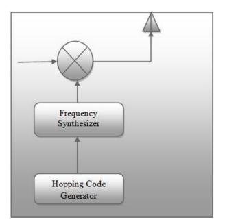
Figure 1. Transmitter for Frequency Hopping Spread Spectrum System
