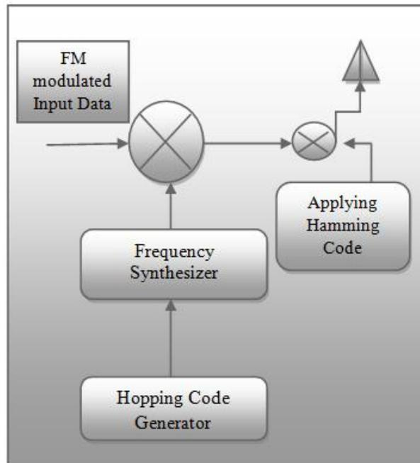
Figure 8. Transmitter for FHSS along Hamming Code
