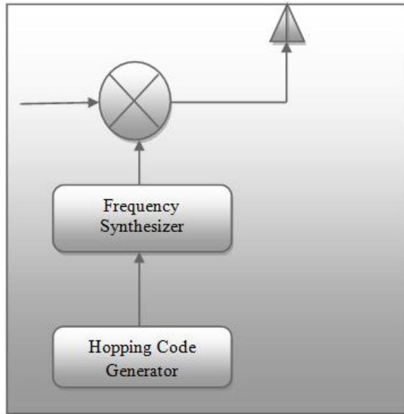
**Figure 1. Transmitter for Frequency Hopping Spread Spectrum System**
