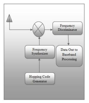
Figure 2. Receiver for Frequency Hopping Spread Spectrum System
