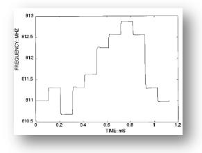
Figure 3. Frequency Hoping: Frequency Vs Time
