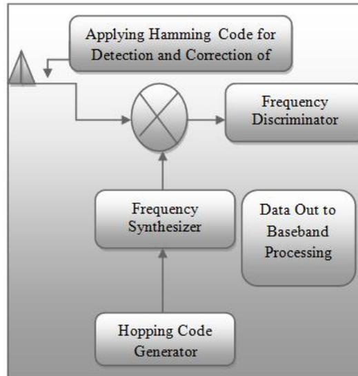
**Figure 9. Receiver for Frequency Hopping Spread Spectrum System using Hamming Code for Detection of Error**
