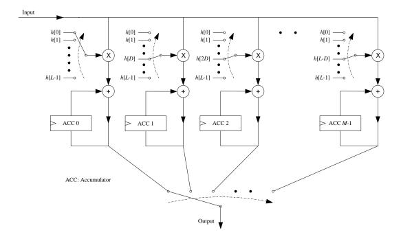
Figure 1. Decimating FIR Filter Architecture of [5]
