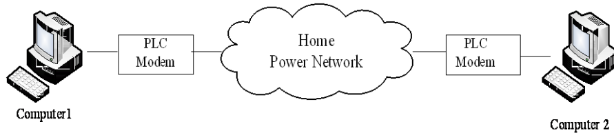
Figure 2. PLC Test Configuration
