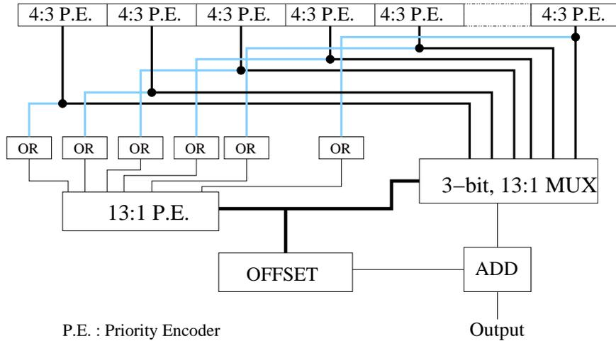
**Figure 3. LOD for FPU Adder/Subtractor**
