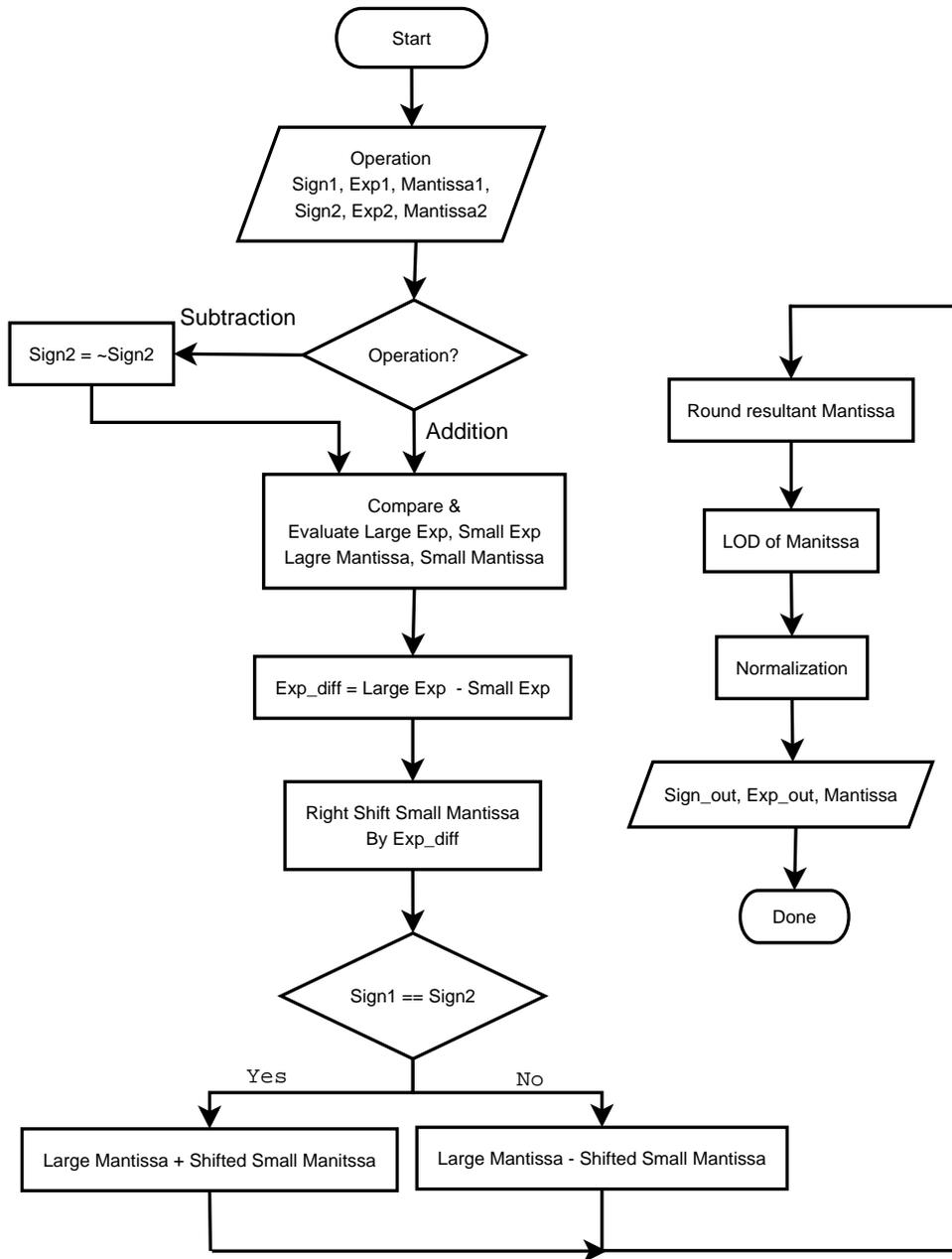
**Figure 1. Flowchart for FPU Adder/Subtractor**
