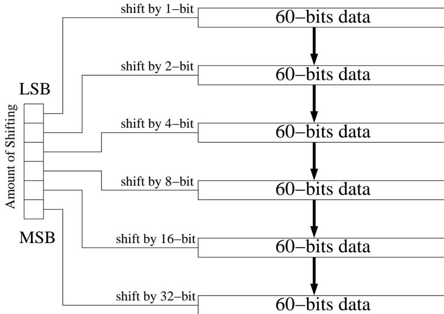
**Figure 2. Dynamic Shifter for FPU Adder/Subtractor**
