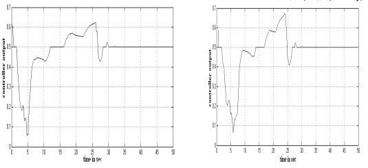
Figure 12. Controller output contribution of the fuzzy block for set point = 70 bar.
