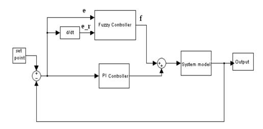
Figure 5. Block diagram of system with Fuzzy assisted PI Controller.
