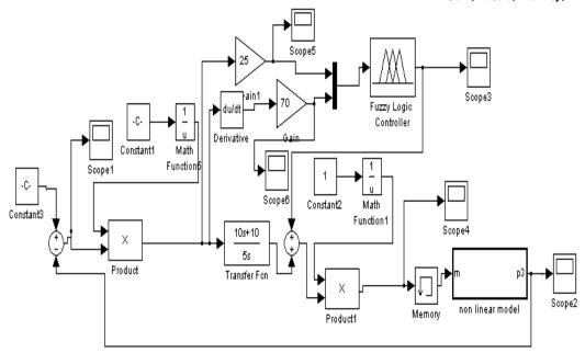
Figure 7. Simulink program of the system with fuzzy assisted PI controller.
