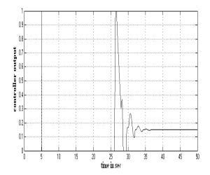
Figure 14. Total controller output of Fuzzy assisted PI controller for set point = 70 bar.
