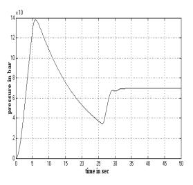
Figure 9. Output response using Fuzzy assisted PI controller for set point 70 bar.
