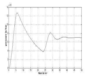
Figure 8. Output response using Pl controller for set point 70 bar .
