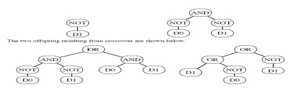
Note that the first offspring above is a perfect solution for the exclusive-or function, namely (OR (AND (NOT D0) (NOT D1)) (AND D0 D1)).
