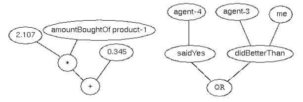
Figure 1. Example of Genetic Programming solution being stored in tree pattern.
