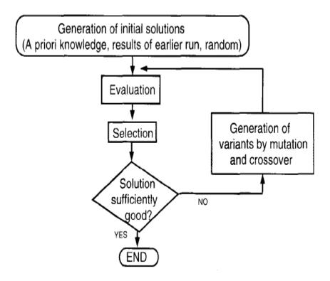
Figure 3. example showing a mechanism in crossover and mutuation to induce an assembler.
