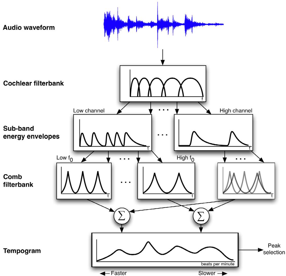
**Figure 2: The processing flow of the beat tracking system. Input audio is divided into sub-bands, downsampled and smoothed, and analyzed by a comb filterbank, the outputs of which are summarized in a “tempogram.”**
