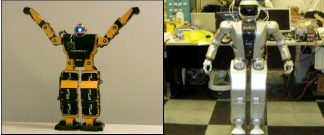
**Figure 1: The Robonova (left) and the Hubo (right)**
