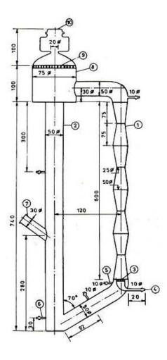
Fig: 2 External Loop Converging-Diverging Tube Air-Lift contactor (CDT-ALC)
