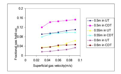
Fig 3 Effect of superficial gas velocity on fractional gas hold-up.
