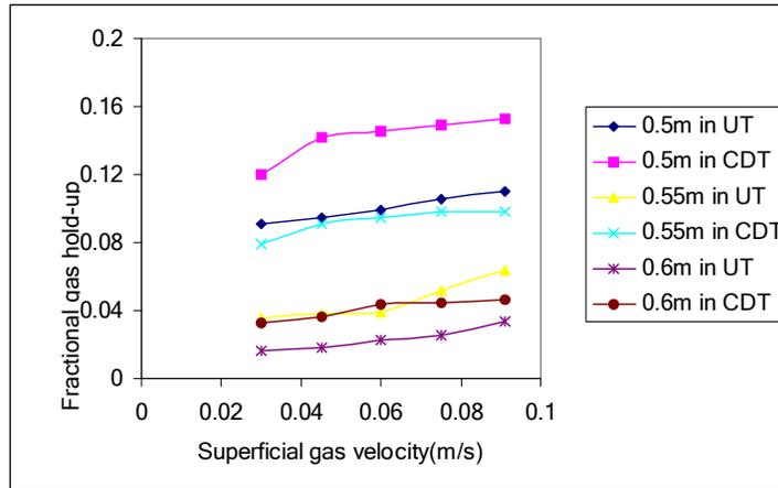
**Fig 3** Effect of superficial gas velocity on fractional gas hold-up.
