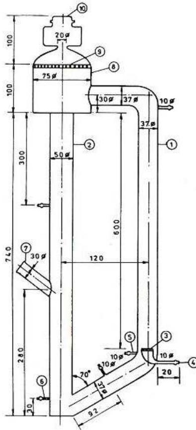
**Fig: 1** Conventional External Loop Uniform Tube Air-Lift Contactor (UT-ALC)
