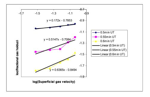
Fig 4 Linear relation between superficial gas velocity and fractional gas hold-up in UT-ALC
