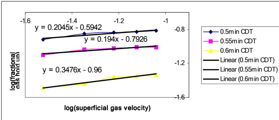
**Fig 5** Linear relation between superficial gas velocity and fractional gas hold-up in CDT-ALC
