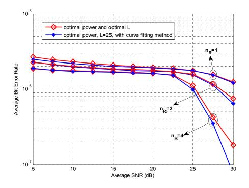
Figure 9. Average bit error rate versus average SNR for optimal power  $\alpha$  and optimal pilot spacing *L* and optimal power with curve fitting method. The number of receive antennas is  $n_R = \{1, 2, 4\}, \tau = 1 \text{ } ms$ , and  $BER_0 = 10^{-5}$ .
