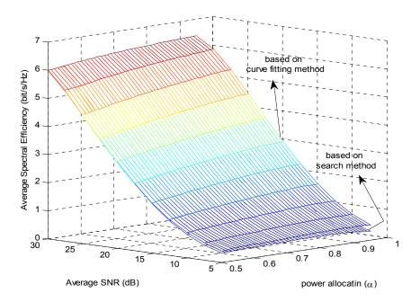
Figure 5. Average spectral efficiency versus average SNR and power allocation  $\alpha$  for both search and curve fitting methods and  $n_R = 2$ ,  $\tau = 1 ms$ , and  $BER_0 = 10^{-5}$ .
