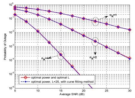
Figure 10. Probability of outage versus average SNR for optimal power  $\alpha$  and optimal pilot spacing *L* and optimal power with curve fitting method. The number of receive antennas is  $n_R = \{1, 2, 4\}, \tau = 1 \text{ } ms$ , and  $BER_0 = 10^{-5}$ .
