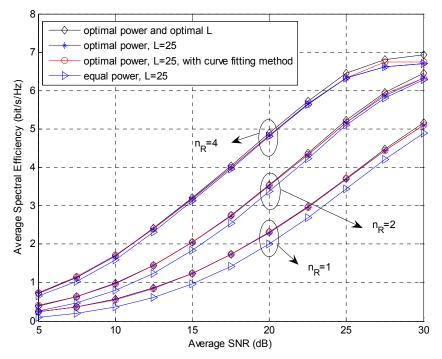
Figure 6. Average spectral efficiency versus average SNR for both optimal parameters and some fixed parameters. The number of receive antennas is  $n_R = \{1, 2, 4\}, \tau = 1 \text{ ms}$ , and  $BER_0 = 10^{-5}$ .
