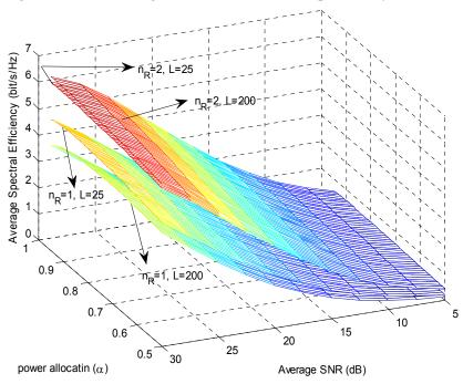
Figure 4. Average spectral efficiency versus average SNR and power allocation  $\alpha$  for different pilot spacing  $L = \{25, 200\}$ . The number of receive antennas is  $n_R = \{1, 2\}, \tau = 1 \text{ ms}$ , and  $BER_0 = 10^{-5}$ .
