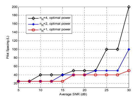
Figure 7. Optimum pilot spacing versus average SNR when power is optimally allocated between the pilot and data symbols. The number of receive antennas is  $n_R = \{1, 2, 4\}, \tau = 1 \text{ ms}$ , and  $BER_0 = 10^{-5}$ .
