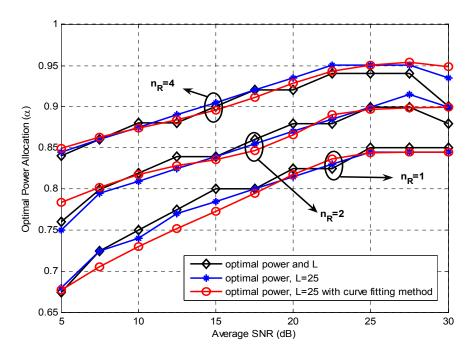
Figure 8. Optimum power allocation to the data symbols versus average SNR when pilot spacing is optimal and L = 25. The number of receive antennas is  $n_R = \{1, 2, 4\}, \tau = 1 \text{ ms}$ , and  $BER_0 = 10^{-5}$ .
