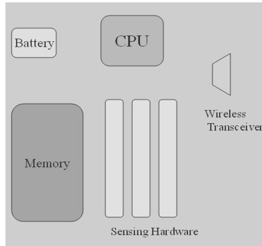
Figure 2. Components of sensor node [4]
