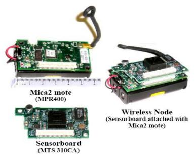
Figure 3. Mica2 mote, sensor board and their combination [3]
