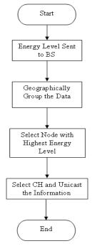
Figure 9. Flow diagram of CH selection
