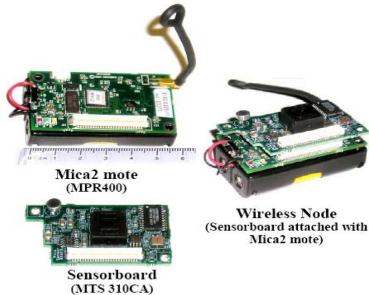
Figure 3. Mica2 mote, sensor board and their combination [3]
