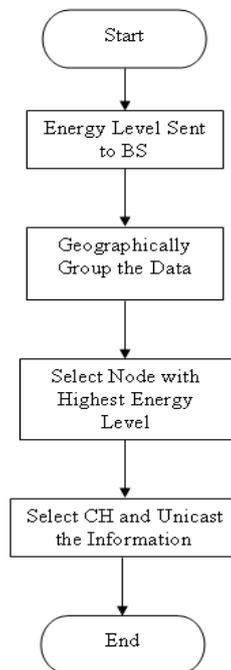
Figure 9. Flow diagram of CH selection
