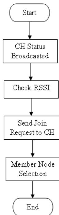
Figure 10. Flow diagram of Cluster Formation
