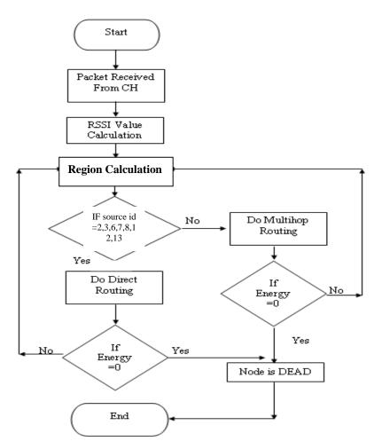
Figure 11. Flow Diagram for Energy Aware Intra Cluster Routing
