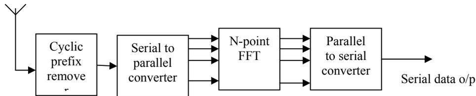
Figure 2. Basic Receiving Section of OFDM
