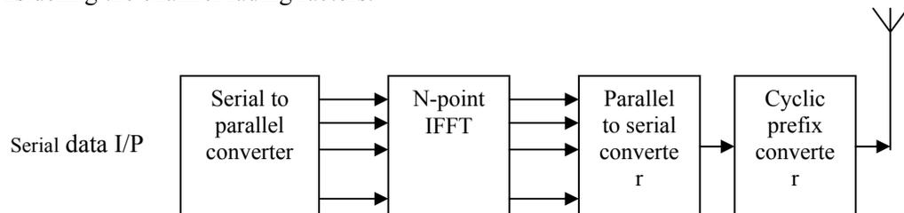
Figure 1. Basic Transmission Section of OFDM
