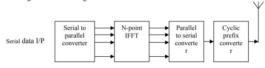
Figure 1. Basic Transmission Section of OFDM
