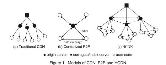
In CDN-level backbone network, the surrogate server is a logical entity and may consist of multiple physical servers or clusters. The request routing in traditional CDN, such as iterative or recursive scheme [6], can be also adopted in HCDN. The existing replica placement strategies [14] can still be used in the CDN-level content distribution.
