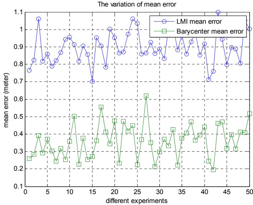
Figure 7. Comparing LMI and barycenter errors across 50 experiments.
