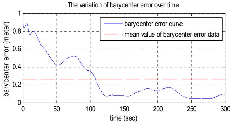
Figure 6. The barycenter error variation curve over waiting time.
