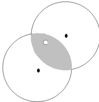
Figure 1. Black dots represent moving nodes knowing their exact position; the white dot represents the user who wants to know his position. Circles represent the maximum range of the moving nodes radio signal.
