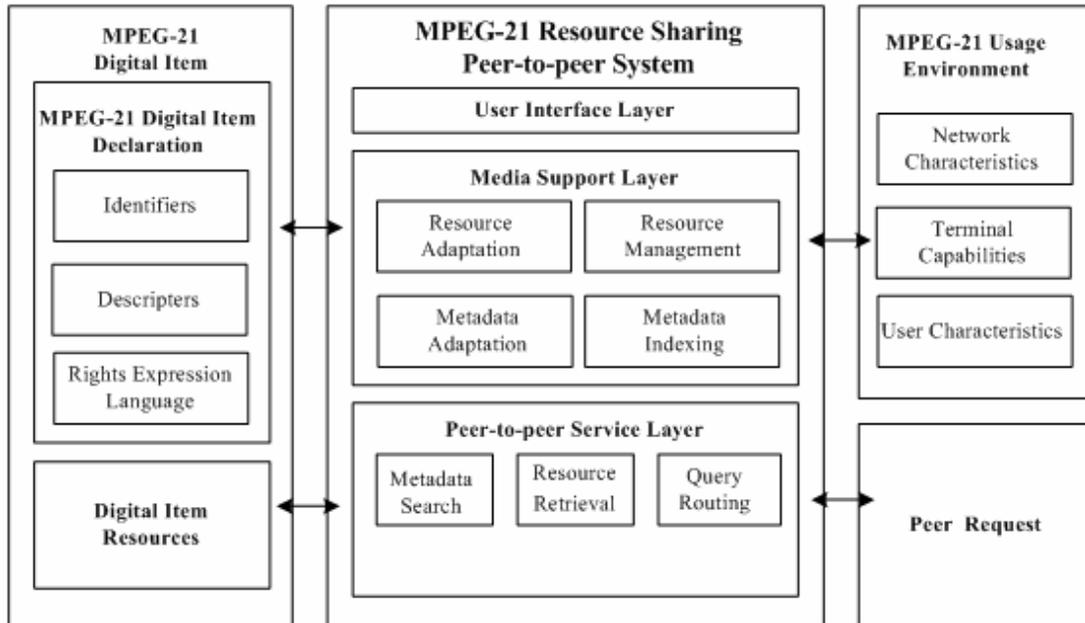
**Figure 2. The abstract system diagram of the proposed P2P architecture.**
