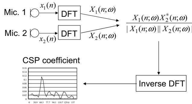
**Figure 3. Estimation of sound source direction by CSP.**
