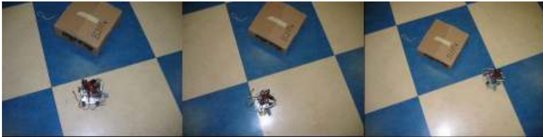
Figure 4. Autonomous Obstacle avoidance using a SMARbot
