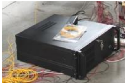
Figure 3. Fiber Grating Sensor Interrogating System
