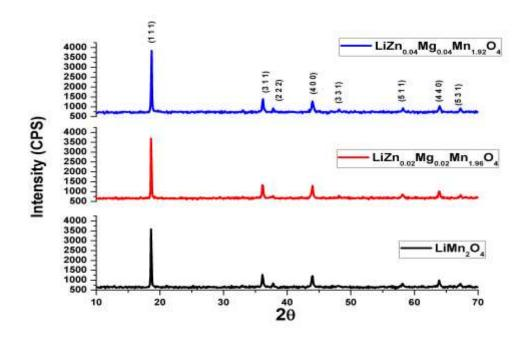
Figure 1. XRD Patterns of  $LiZn_xMg_yMn_{2-x-y}O_4$  (x = y = 0, 0.02, 0.04)
