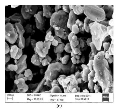
Figure 2. (a) to (c): SEM Images of  $LiZn_xMg_yMn_{2-x-y}O_4$  (x = y = 0, 0.02, 0.04)
