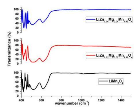
Figure 3. FT-IR Images of  $LiZn_xMg_yMn_{2-x-y}O_4$  (x = y = 0, 0.02, 0.04)
