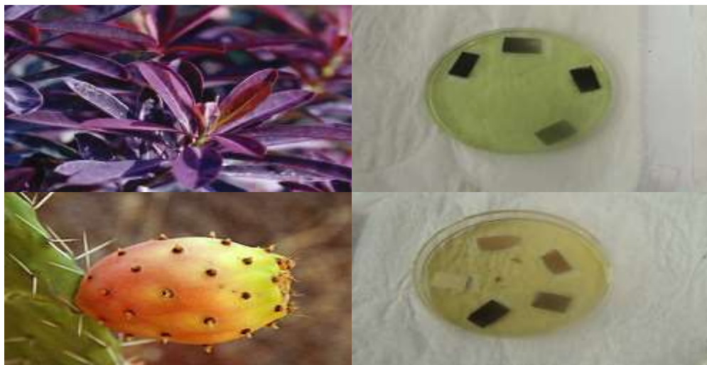
Figure 2. E. Amygdaloides Leaf and Opuntia Ficus Indica Fruit then Soaked with Working Electrode in the Extracted Dye
