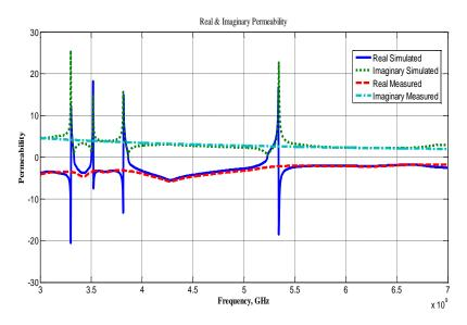
Figure 5. Simulated and Measured Permeability vs. Frequency, GHz
