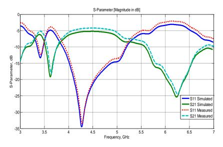
Figure 4. Simulated and Measured S11 and S21 Parameter
