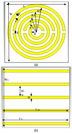
Figure 1. (A) Circular SRR Top View, (B) Wires Back View
