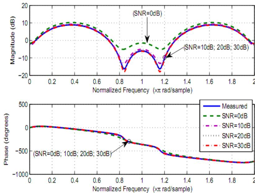
**Figure 3. Estimated Magnitude and Phase of the Model 2, for  $N = 2000$  and Different SNR**
