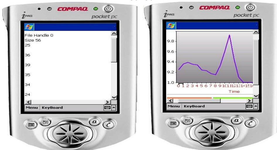
Figure 6. a) Mobile with read option selected; b) Mobile with draw graph option
