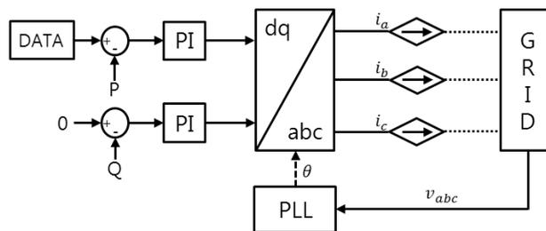
Figure 2. PV/wind-turbine hybrid system model based on equivalent current model
