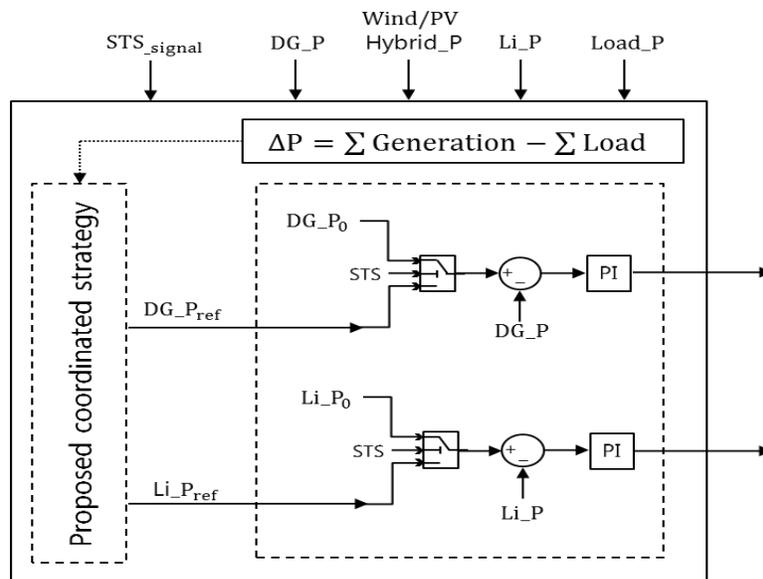
**Figure 9. shows configuration of the proposed coordinated frequency controller**
