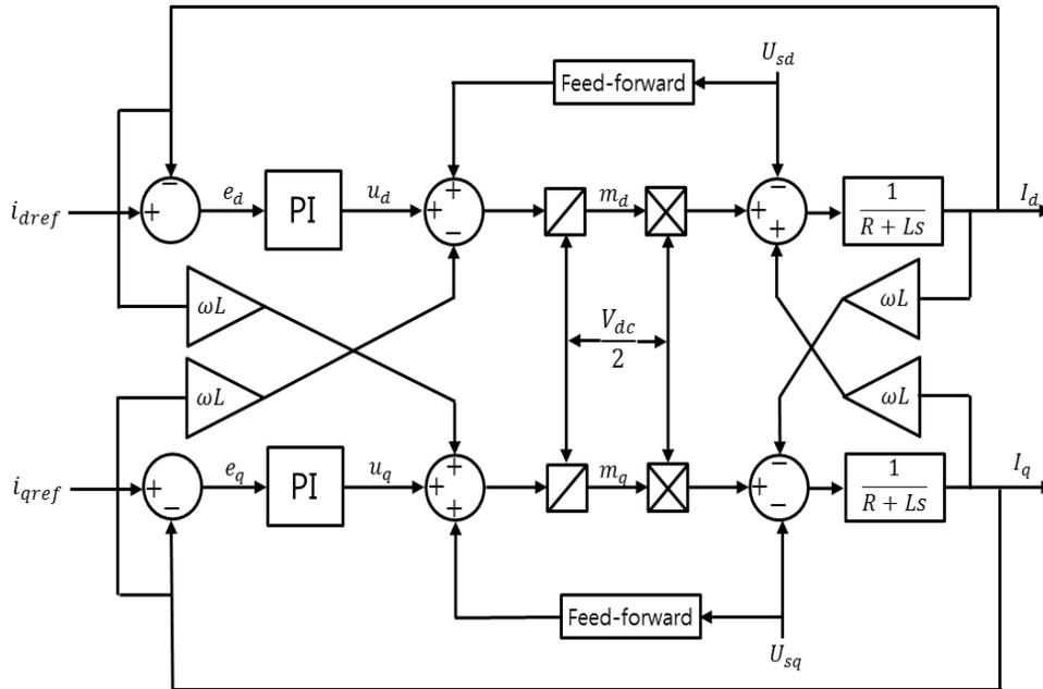
**Figure 6. The control block diagram of current controller**
