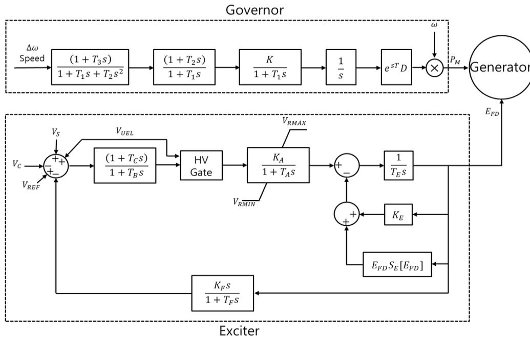
Figure 1. Diesel generation system model
