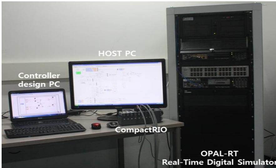
Figure 11. Developed HILS system and tested coordinated controller
