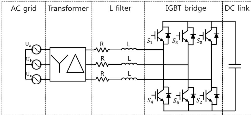
**Figure 4. The structure of 2-level VSC**
