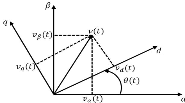
**Figure 5.  $\alpha\beta$ -frame and dq-frame coordinated system**
