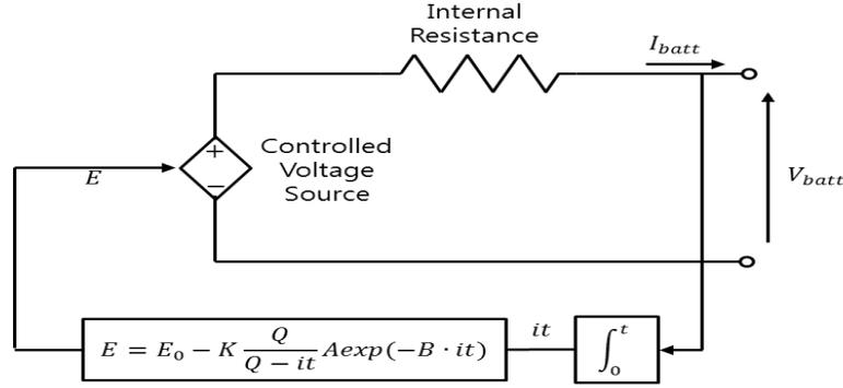
**Figure 3. The battery model**
