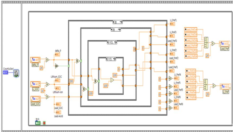
Figure 10. Designed coordinated controller using CompactRIO
