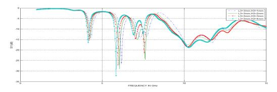
b) Effect of H<sub>3</sub> on return loss at L<sub>3</sub>=3mm
