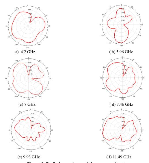
Figure 9. Radiation patterns of the proposed antenna
