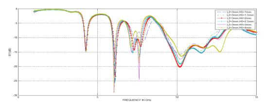
(b) Effect of H<sub>5</sub> on Return loss at L<sub>2</sub>=3mm
