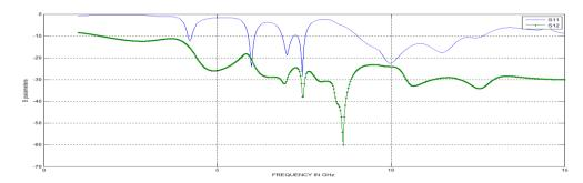
Figure 6. S parameters of proposed slotted Fork shaped microstrip patch antenna
