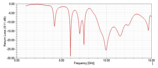
Figure 2. Return loss of the proposed antenna
