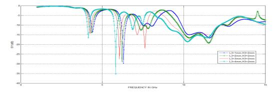
(a) Effect of  $L_3$  on return loss at  $H_3$ = 2mm.
