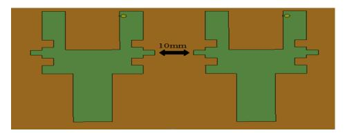
Figure 5. A two element MIMO system using proposed slotted Fork shaped antenna
