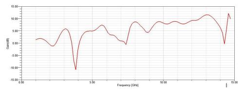
Figure 10. Gain plot of the proposed antenna
