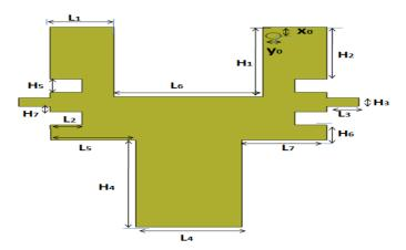
Figure 1. Proposed slotted Fork shaped microstrip patch antenna
