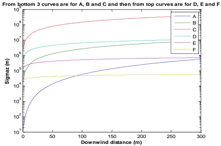
Figure 3 Vertical Dispersion Coefficient ( $\sigma_z$ )
