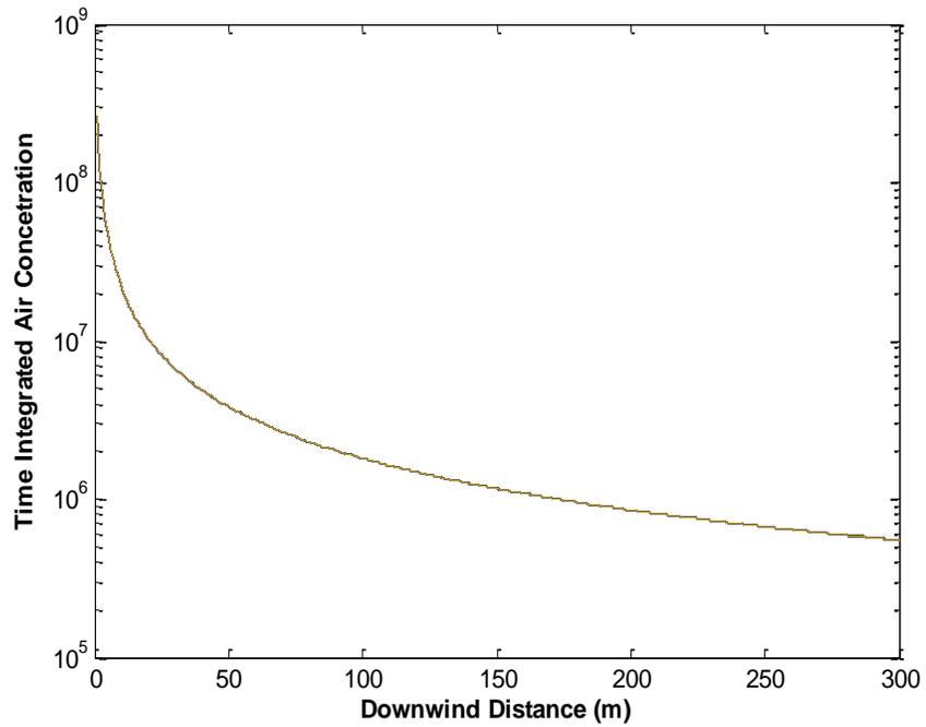
**Figure 5. Time Integrated Air Concentration for an Elevated Release and with Plume Rise for Weather Category 'F'**
