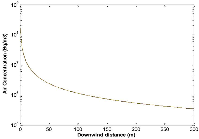
**Figure 4. Time Integrated Air Concentration for an Elevated Release and without Plume Rise for Weather Category 'F'**
