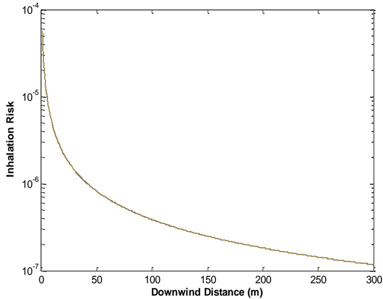
**Figure 6. Inhalation Risk at Various Downwind Distances with Elevated Release and Plume Rise for Weather Category 'F'**
