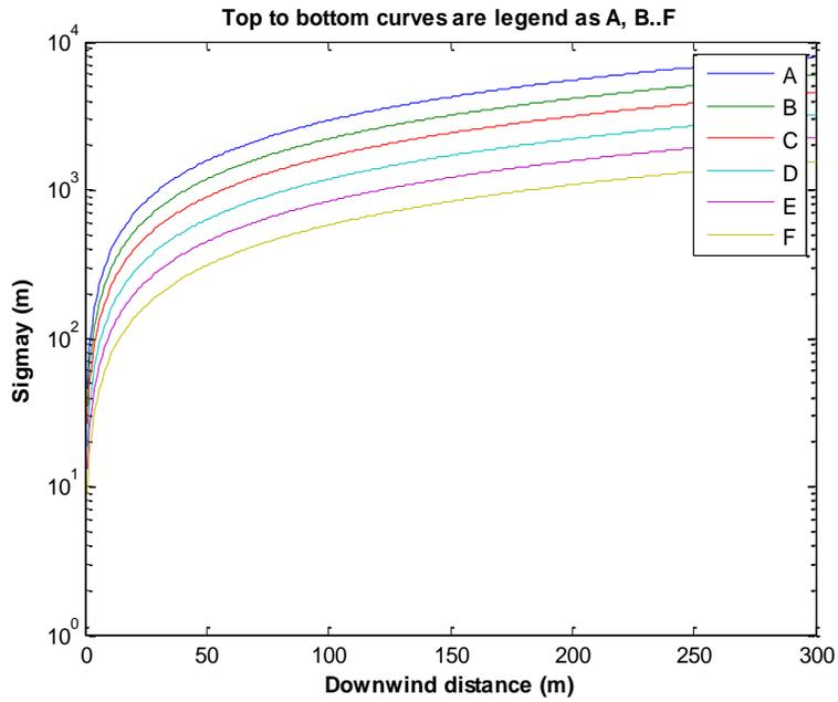
Figure 2. Horizontal Dispersion Coefficient ( $\sigma_y$ )
