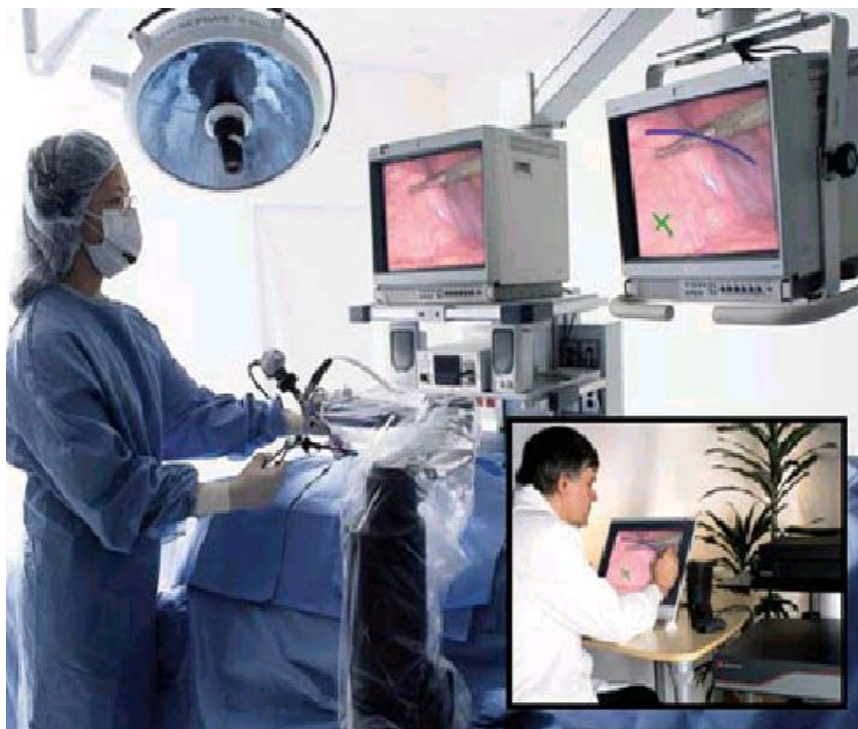
Figure 2. The SOCRATES™ Robotic Telecollaboration system used for the proposed network-based telemedicine (surgical) service: The system can give the remote surgeon direct access to the operative environment and key patient information. The system also provides the remote surgeon with uncompromised operative visualization and the ability to remotely control the position of the endoscope. Operation in OR collaborated with surgical telementoring using SOCRATES™ system (large) and surgical specialist's dialogue with a telestration feature for annotation of a shared video image at remote site (inset). Photo Courtesy of the Intuitive Surgical Inc.
