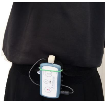
Figure 2. Wireless Triaxial Accelerometer attached to the Waist
