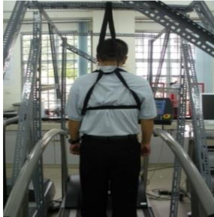
Figure 3. Treadmill Walking Supported by the Safety Belt
