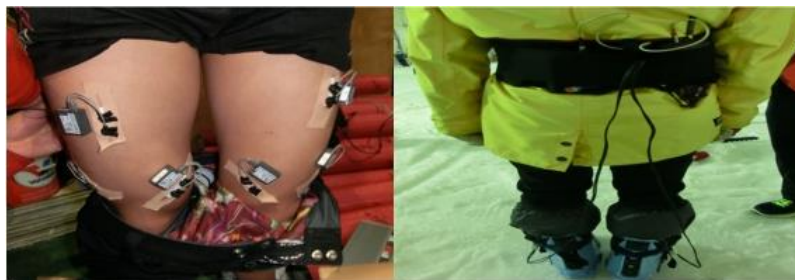
Figure 1. Views of the Subject Wearing EMG Electrodes and the Pedar Sensor
